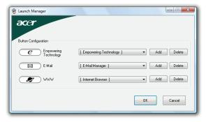
Launch Manager allows you to set the four easy-launch buttons located above the keyboard. **"Easy-launch buttons" on page 26** for the location of the easy-launch buttons.
