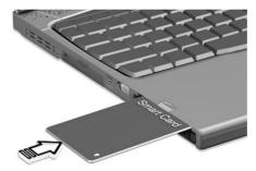
To remove the SmartC ard press the SmartC ard eject button (a) and remove the SmartC ard (b) as shown in the illustration below.
