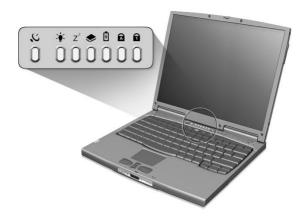
The Power and Sleep status ic ons are visible even when you close the display coverso you can see the status of the computer while the cover is closed.
