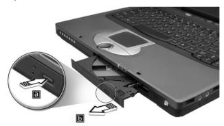
When the power is off, you can eject the drive tray using the emergency eject hole. See page 49.
