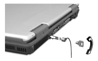
Wrap a computer security lock cable around an immovable object such as a table or locked drawer handle. Insert the lock into the notch and turn the key to secure the lock. Some keyless locks are also available.
