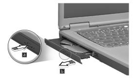
When the power is off, you can eject the drive tray using the emergency eject hole. See page 50.
