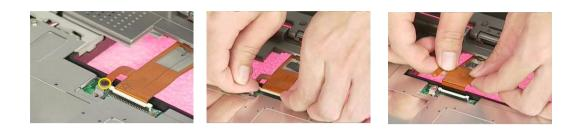
3. Remove the two screw holding the LCD FPC cable on the bottom.
