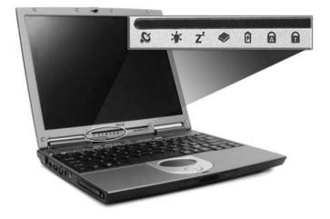
The Wireless, Power and Sleep status indicators are visible even when the display is closed.
