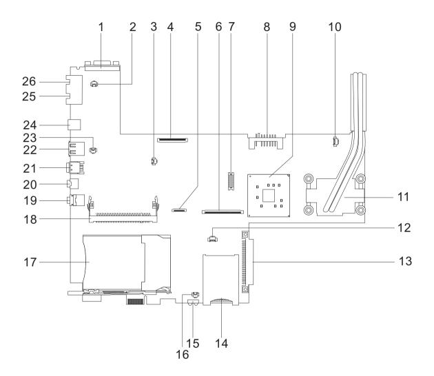
External Display Port 1 2 Modem Cable Connector 3 Speaker Connector 4 LCD FPC Connectors 5 **Touchpad Board Connectors** 6 Keyboard Connector 7 Modem Board Connector 8 **Battery Connector** 9 North Bridge 10 Fan Connector CPU 11 12 **RTC Battery Connector**
