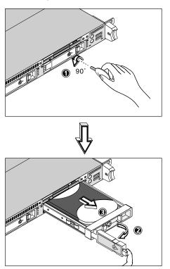
3 Remove the four tray screws to open the drive tray. Keep the screws for later use.
