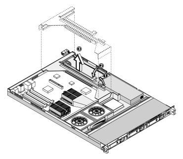
3 Gently pull out the metal bracket with the riser card from the mainboard.
