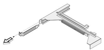
4 Remove the expansion card bracket. Save the screw for later use.
