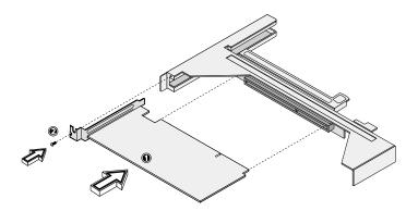
7 Reinstall the metal bracket with the riser card into the mainboard system and secure it with the two screws you have previously removed.
