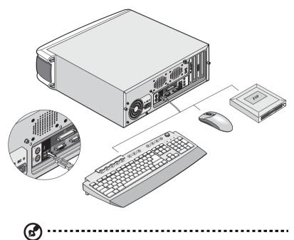
**Note:** Some USB devices have a built-in USB port which allows you to connect or daisy-chain more USB devices.
