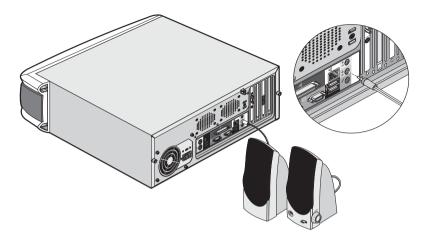
audio line-in device: connects to the Audio-in/Line-in jack (\*\*) (light blue jack) located on the rear panel of your computer
