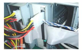
8. Disconnect the bezel LED cable and the ODD power cable.
