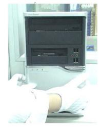
3. Rail the holder shown below, then take the ODD out from the chassis.
