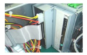
**10.** Disconnect the HDD data cables and power cables from the rear of the HDD.
