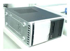
2. Release the lock handle and slide the left cover out.
