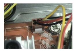
2. Release the CPU Cooler latch then remove it.
