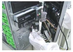
3. Release the ODD rails and disassemble the two ODDs.
