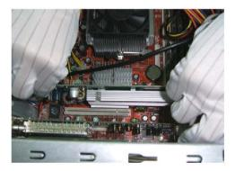
3. Pull out the CD\_IN cable from TV tuner card.
