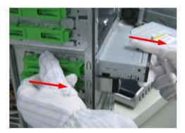
5. Release the rail and remove the Card Reader.
