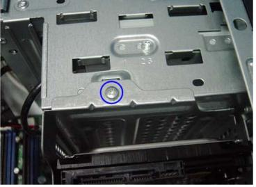
**b.** Lift the bracket up and turn it over.
