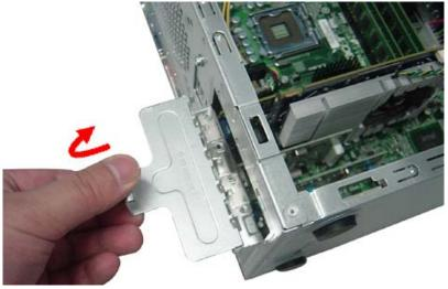
3. Use a figer to press the clip, and the same time Gently pull the card to remove it from the mainboard.
