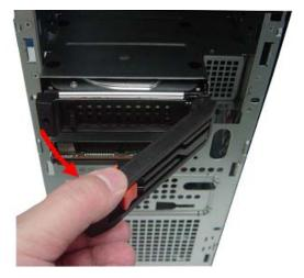
2. Slide the removable HDD tray out of the removable HDD bracket.
