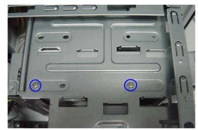
d. Remove the removable HDD out of the chassis.
