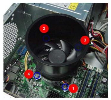
2. Lift the heat sink fan assembly away from the mainboard.
