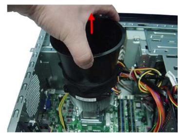
**3.** Lay down the heat sink fan assembly, in an upright position, on top of the optical drive, as shown below, then disconnect the fan cable from the mainboard.
