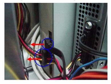
2. Disconnect the other end of the data cable from the mainboard.
