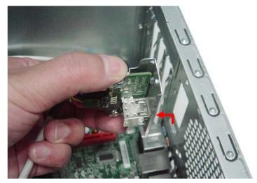
5. Remove the two screws that secure the USB board to the bracket.
