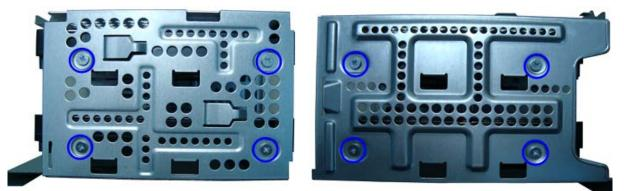
**b.** Slide the HDD out of the bracket.
