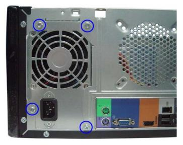
3. Lift the power supply module out of the chassis.
