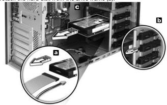
Insert the new hard disk into the frame (a).
