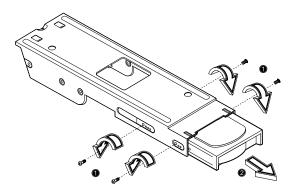
6 Insert the new hard disk into the frame and secure it with four screws. .
