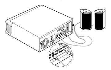
audio line-in device: connects to the Audio-in/Line-in jack (\*\*)
