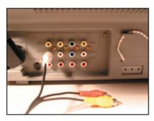
**9.** Plug **one Red RCA Plug** into the **Red Right("R") Audio Out Port** on the rear panel of the Player.
