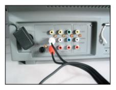
**11.** Plug **one Yellow RCA Plug** into the **Yellow Video Out Comp Port** on the rear panel of the Player.
