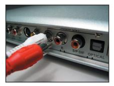
**10.** Plug the other end of the **Red RCA Plug** into the **Red Audio In Port** on the television or stereo.
