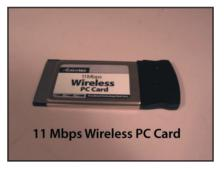
**14.** Remove the cover from the **wireless card slot** on the side of the Player and plug the **Wireless Card** into the slot.
