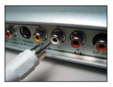
**8.** Plug the **other White RCA Plug** into the **White Audio In Port** on the television or stereo.
