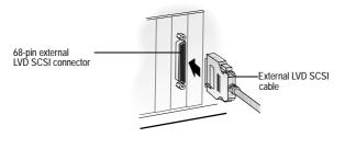
**2** Connect the other end of the cable to a SCSI connector on the back of an external device. If you are installing only one external device, terminate the device and skip to Step 4.
