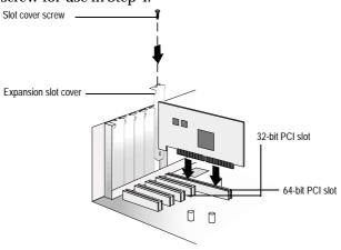
Computers may have vertical or horizontal expansion slots. Refer to your computer manual to locate the PCI/PCI-X slots. If your computer is a tower model, lay it on its side to allow for easier installation of the Adaptec SCSI Card 29320A.
