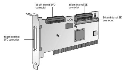
Although the Adaptec SCSI Card 29320A is a 64-bit PCI/PCI-X card, it also works in a 32-bit PCI slot. When installed in a 32-bit PCI slot, the card automatically runs in the slower 32-bit mode.
