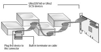
Note: Internal Ultra320/160 and Ultra2 SCSI devices come from the factory with termination disabled and cannot be changed. Proper termination is provided by the terminator at the end of the LVD SCSI cable.
