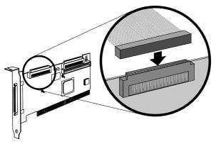
**3** Plug the internal Ultra320/160 and Ultra2 SCSI devices to the other cable connectors, starting with the connector at the terminated end of the cable.
