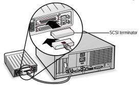
**3** Connect the other external SCSI devices by linking each device to the previous one, as shown below. Terminate only the device at the end of the chain.
