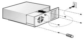
**3** Locate an unused 64-bit PCI/PCI-X expansion slot and remove the expansion slot cover. If the computer does not have a 64-bit slot, you can install the card in a 32-bit PCI slot. The Adaptec SCSI Card 29320A supports both 5V and 3.3V 64-bit slots. (The expansion slot must be compliant with PCI Rev. 2.1 or PCI-X Rev. 1.0 and must support Bus Mastering.) Save the slot cover screw for use in Step 4.
