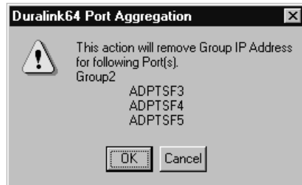
Figure 8-12. This message appears when you add ports with IP Addresses to a new group.
