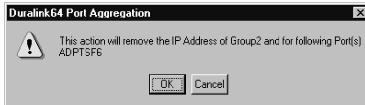
Figure 8-13. This message appears when you add ports with IP Addresses to Group2 with an existing IP Address.
