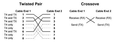
A simple network can be made by connecting a Quartet server directly to four workstations via crossover cables.
