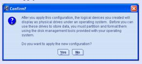
Adaptec Storage Manager builds the logical drive(s). The configuration is saved on the Adaptec controller and on the physical drives.
