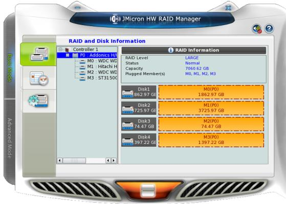
In the event of a drive failure, the Jmicron RAID Manager will present a dialog box such as the one shown below, even if it is currently minimized to the system tray:
