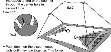
• Connect the tent to frame by pulling the shock-corded loops, at the peaks of the tent, over the junction tubes. Snap tent clips to the poles.
