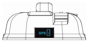
In Self-Test, the display illustrates the test result of each step with " $\sqrt{}$ " indicating a pass and "X" indicating a failure. There are a total of five tests, plus a battery check. If all tests pass, SELF-TEST PASS will be displayed at the end of the Self-Test mode. This will be followed by the GPS coordinates horizontally scrolling through the display, provided the beacon has successfully downloaded an external GPS location. See Appendixes B through E for details about display messages.
