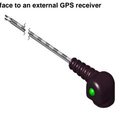
If you have a Category I beacon and bracket, the connector is at the end of the black lead wire plugs into the beacon via the bezel on the top of the beacon. See the location of the GPS interface in previous figures ("Anatomy of your beacon", page 7 and "Top View", page 8). It is important to seat the connector completely in the bezel for an operational connection.
