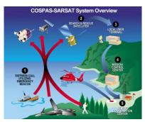
within the view of the satellite, as well as being stored for later transmission to other LUTs.
