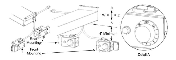
1. Use 88904 (screw), 89056 (washer), and 88921 (nut) to mount bracket. Place bracket (70402017) around shelving pole on the inner side of the shelving unit. Screw bracket (70402018) to bracket (70402017) around shelving pole on the outer side of the shelving unit. The bracket will allow the remote box inner side to align with the front side of the food warmer
