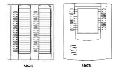
The module connects to the right side of the 6757i CT RP phone via an RJ-45 connector.
