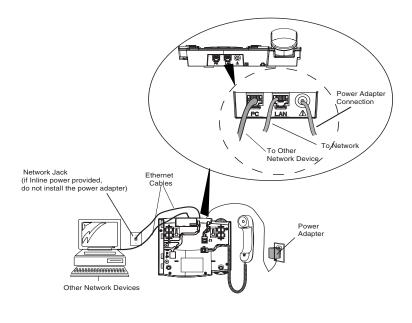
**Note:** The **PC** jack on the 6757i CT RP does not supply inline power onto other network devices. All Ethernet cables used must be category 5/5e straight-through cables, such as the cable provided with your phone
