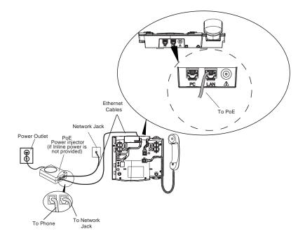
**Note:** You should connect the power supply to a surge protector or power bar. All Ethernet cables used must be category 5/5e straight-through cables, such as the cable provided with your phone.
