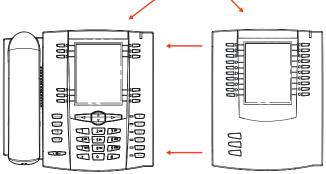
The M670i provides 36 additional softkeys on a 6757i CT RP Phone. The M675i provides 60 additional softkeys.
