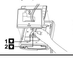
Attach the line cord to jack number 2 and the other end to the modem or fax machine. This line cord is not supplied with the telephone.
