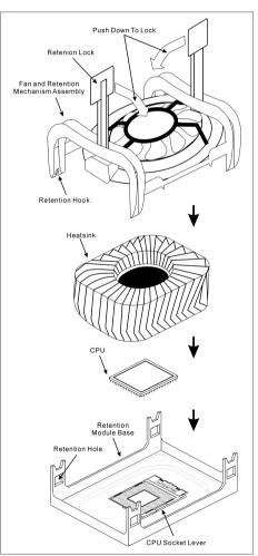
5. Push down the Retention Lock at both sides of the Fan and Retention Mechanism Assembly to lock up together with the Retention Module Base.
