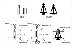
studs. If the holes line up and there are only slots, you can only attach with spacers. Take the tip of the spacers and insert them into the slots. After doing this to all the slots, you can slide the board into position aligned with slots. After the board has been positioned, check to make sure everything is OK before putting the chassis back on.
