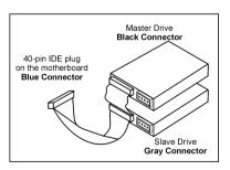
**NOTE:** Make sure to configure the "Master" and "Slave" relation before connecting two drives by one single ribbon cable. The red line on the ribbon cable must be aligned with pin-1 on both the IDE port and the hard-drive connector.
