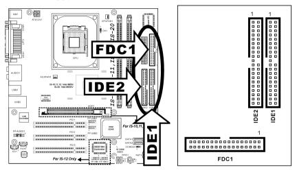
The FDC1 connector connects up to two floppy drives with a 34-wire, 2-connector floppy cable. Connect the single end at the longer length of ribbon cable to the FDC1 on the board, the two connectors on the other end to the floppy disk drives connector. Generally you need only one floppy disk drive in your system.
