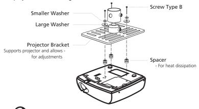
**Note:** It is recommended that you keep a reasonable space between the bracket and the projector to allow for proper heat distribution. Use two washers for extra support, if deemed necessary.
