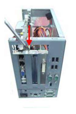
Step 6 Close the top cover back to the chassis and fasten all screws.
