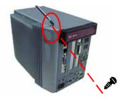
Step 4 After opening the top and side covers, you can locate the CPU socket and heatsink as marked. Align pins of the CPU with pin holes of the socket. Be careful of the CPU's orientation that you need to align the arrow mark on the CPU with the arrow key on the socket. Place the CPU into the socket, and use a screwdriver to lock it onto the socket.
