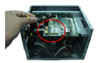
Step 6 Place the CPU Heatsink on the CPU, and lock it by pushing down the fixing buttons.
