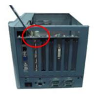
Step 4 Locate the PCI or PCIe slots from the side.
