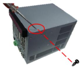
Step 4 Open the top cover and locate the two Hard Disk Drives from the side.
