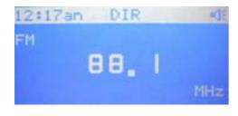
Press the CH +/- buttons to change FM frequency in 100kHz steps; press select
