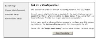
4. The "Actiontec DSL Gateway Setup Page" screen appears. Using the Internet Service Provider (ISP) worksheet, enter the following information: ISP Protocol (select RFC1483 Bridged, RFC1483 Routed, PPPoA, or PPPoE by clicking in the appropriate circle), ISP Username, ISP Password (in the appropriate text boxes).
