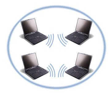
Ad hoc mode is also called peer-to-peer mode or independent basic service set (IBSS). This mode is useful when communicating among many computers locally without the need to connect to printers or file servers on a wired LAN.
