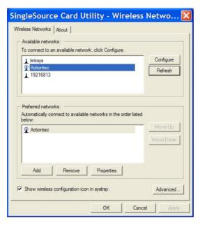
To configure the SSID or name of a wireless network, highlight the name ("Actiontec" in the figure above, for example) and click **Configure**. To automatically connect to a particular network every time the Adapter searches for a network, click **Add**, select the network, and, when the network name appears in the "Preferred networks" list box, select it. Using the "Move Up" button, make sure the selected network appears at the top of the list.
