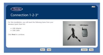
**3.** Plug the smaller end of the USB cable into the port on the front of the Adapter, then click **Next**.
