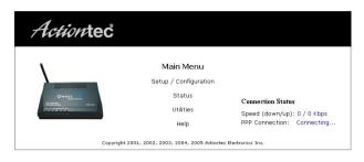
**3.** In the "Set Up/Configuration" screen, select **Alternative Setup** from the menu on the left side.
