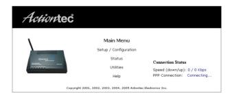
**Note:** If the Main Menu screen does not appear, make sure the Ethernet cable is properly connected.
