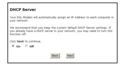
Actiontec strongly recommends leaving the DHCP Server option **On**. If the DHCP Server option is **Off**, ensure the IP addresses of the networked computers are on the same subnet as the IP address of the Modern. For more information, see "DHCP Server Configuration."
