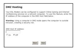
DMZ hosting is used to support online gaming and Internet conferencing services. These programs usually require multiple open ports, making the network accessible from the Internet. DMZ hosting symbolically places the DMZ host computer outside of the Modem's network. Actiontec recommends activating DMZ hosting only as long as necessary.
