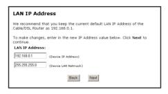
The values in the "LAN IP Address" and "Netmask" text boxes are the IP address and Subnet mask of the Router as seen on the network. These values can be modified for your LAN network, but Actiontec recommends keeping the default factory settings (IP address 192.168.0.1; Subnet mask 255.255.255.0).
