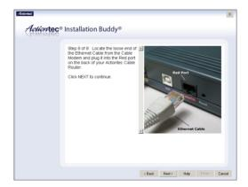
**21.** If connecting via USB, plug the other end of the **Ethernet cable** into the **Ethernet port** on the cable modem, then click **Next**.
