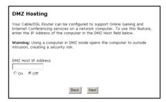
DMZ hosting is used to support online gaming and Internet conferencing services. These programs usually require multiple open ports, making the network accessible from the Internet. DMZ hosting symbolically places the DMZ host computer outside of the Router's network. Access to the network resources while DMZ hosting is active is blocked. Actiontec recommends activating DMZ hosting only as long as necessary.
