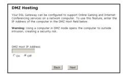
DMZ hosting is used to support online gaming and Internet conferencing services. These programs usually require multiple open ports, making the network accessible from the Internet. DMZ hosting symbolically places the DMZ host computer outside of the Gateway's network. Actiontec recommends activating DMZ hosting only as long as necessary.
