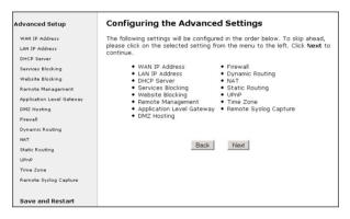
**Note:** To save changes made in any of the Advanced Setup screens, click **Save and Restart** at the bottom of the gray menu on the left side of the screen.
