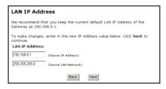
The values in the "Device IP Address" and "Device LAN Netmask" text boxes are the IP address and Subnet mask of the Gateway as seen on the network. These values can be modified for your LAN network, but Actiontec recommends keeping the default factory settings (IP address 192.168.0.1 Subnet mask 255.255.255.0).
