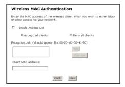
This feature allows the user to control the wireless LAN network by denying or allowing wireless access by specifying the MAC address of the wireless client(s) allowed or denied access on the wireless network.
