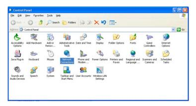
**4.** In the "Network Connections" window, double-click **Local Area Connection**. A number may be displayed after the Local Area Connection. If more than one Local Area Connection is listed, locate the one that corresponds to the network card installed in your computer by finding the name of the network card in the "Device Name" column.
