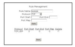
In this screen, the user can create a custom set of rules for a game or application not listed in the Application Level Gateway screen. Enter the "Rule Name," "Protocol," "Port Start," "Port End," and "Port Map" in the appropriate text boxes, then click Apply. The rules are summarized at the bottom of the screen, and the rule set will appear in the Application Level Gateway screen after clicking **Back**.
