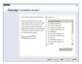
**Manual Setup** - If the Auto Detect and Select from a list are not successful, or the user knows how to configure VPI/VCI and Encapsulation settings, click in the "Manual Setup" box, then click **Next**.
