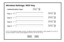
**Authentication Type** - There are three authentication types: Open, Shared, and Both. Open authentication allows any wireless-enabled device to recognize the network, even if the WEP key is invalid. Shared allows only wireless-enabled devices with the correct WEP key to recognize the network.
