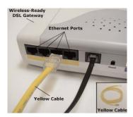
**2.** Plug the loose end of the **Yellow Cable** into the **Ethernet Port** on the back of the computer.
