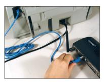
**3.** Plug the Power cord back into the Power port of the Print Server.
