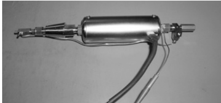
Figure 42 Proper Alignment of the Burner
