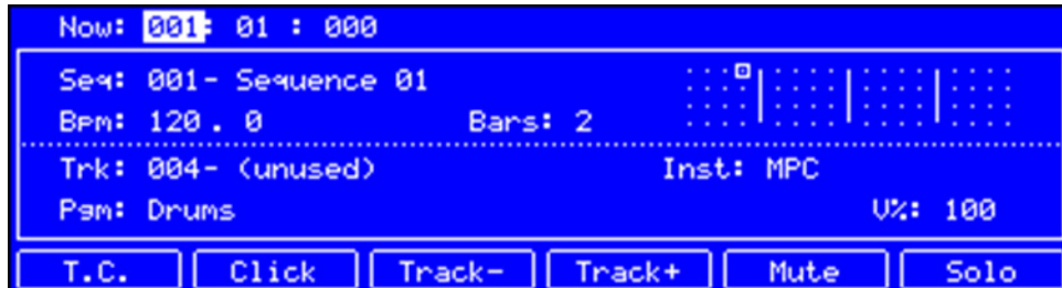
The Main section in the display of the MPC hardware
