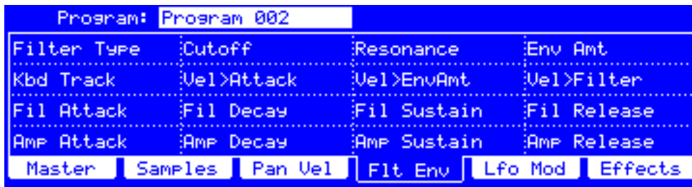
The Filter and Envelope display of the MPC hardware
