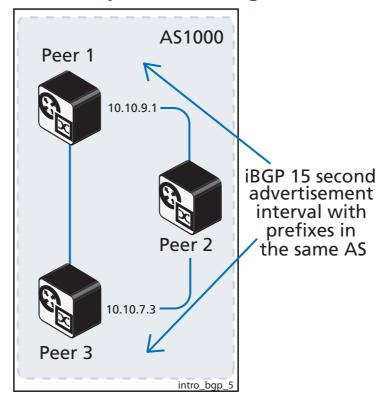
How to adjust the AS origination interval
