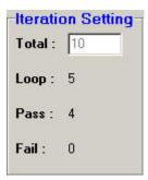
Input the total number of times the test to be run, including total loop, loop for current, pass time and fail time.
