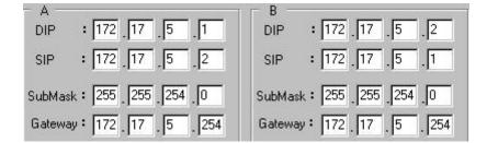
Set up Port A and Port B's IP addresses. Port A's DIP (B) is the same as Port B's SIP
