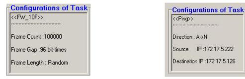
Showing information of current parameters for Frame test including server address, frame length, frame count, frame gap, and for Ping test including direction, source IP and destination IP.
