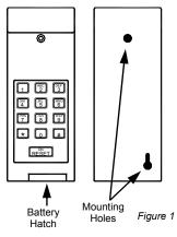
bottom screw. Install the screw leaving the head of the screw approximately 1/8 inch out from the wall. Slide the keypad over the screw and mark the position of the top hole. Remove the keypad and drill the top hole. Slip the keypad back over the exposed screw and finish mounting by installing the top screw. Refer to Figure 1.
