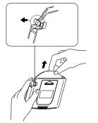
To remove discs from the CD magazine, first find the lever corresponding to the CD you would like to remove. Push the lever away from the magazine. The disc will come halfway out from the CD magazine. Carefully grasp the edge of the disc as shown and remove.
