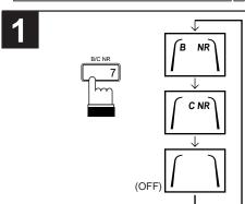
Press the 7 (B/C NR) button in the tape mode to select the Dolby B NR or C NR to play a Dolby B NR or C NR encoded tape respectively. The B or C indicator appears in the display to show your selection. A reduction in tape hiss should also be noticed, with a properly encoded tape.
