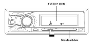
Press any one of the 6 positions on the GlideTouch bar to which a function has been assigned in the guide display. For example, to select ON, press the GlideTouch bar directly below where ON is indicated in the guide display. The manual expresses this as follows: "Change the setting by pressing the GlideTouch bar below either the ON or OFF function indicators."
