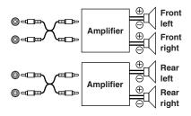
**POWER-IC ON**: The speakers are driven by the built-in amplifier.
