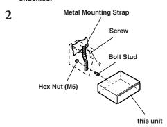
When your vehicle has the Bracket, mount the long hex bolt onto the rear panel of the CDA-9855R/CDA-9853R and put the Rubber Cap on the hex bolt. If your vehicle does not have the Mounting Support, reinforce the head unit with the metal mounting strap (not supplied). Connect all the leads of the CDA-9855R/CDA-9853R according to details described in the CONNECTION section.
