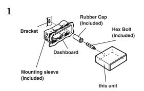
Slide mounting sleeve from main unit (see "Removal" on this page). Slide the mounting sleeve into the dashboard and fix it with the metal shackles.
