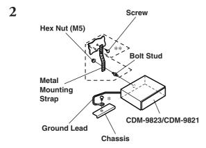
Reinforce the head unit with the metal mounting strap (not supplied). Secure the ground lead of the unit to a clean metal spot using a screw (\*) already attached to the vehicle's chassis.
