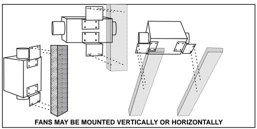
anchors are recommended. The rubber grommets provide vibration isolation.
