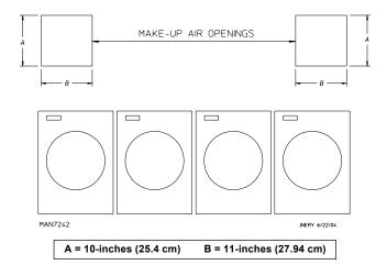
EXAMPLE: For a bank of 4 M31SL dryers, 2 unrestricted openings measuring 10-inches by 11-inches (25.4 cm by 27.94 cm) are acceptable.
