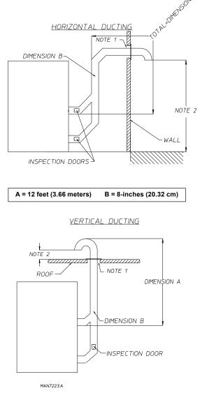
NOTE 1 Opening from combustible materials must be 2-inches (5.08 cm) larger than the duct (all the way around). The duct must be centered within this opening.
