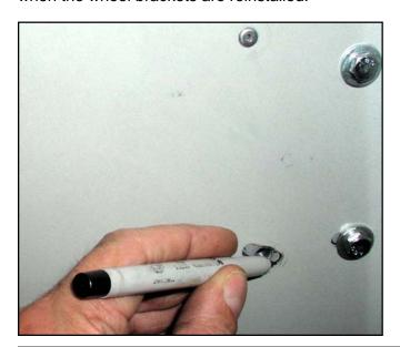
Adjust the tumbler position by loosening the three bolts and forcing the wheel assembly toward the center of the dryer to raise the tumbler and to move it away from the side. A large screwdriver can provide the necessary leverage. Adjustment of the front of the tumbler is made by equalizing the gap on the top, bottom, left and right by moving the wheel assemblies.
