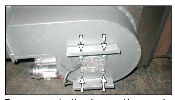
To remove motorized impellor assembly, remove lint housing cover, lint screen, and the four screws shown with arrows. Pull the motorized impellor assembly out through the opening.
