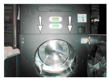
Tilt the top of the panel out, disconnect electrical connection to computer panel, lift panel and unhook support brackets.
