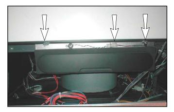
Unplug two connections on the exhaust hi-limit at the left of the lint box. The lint box may now be pulled out through the front of the dryer.
