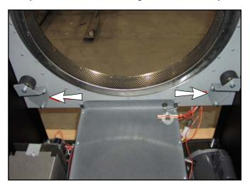
The left rear wheel assembly can be removed with just the back guard removed. The rear right wheel requires removing the back guard, heat duct, and oven. Be sure to mark the position of rear wheel brackets prior to removal (refer to **page 7**).
