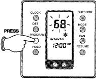
*Step 5:* Press the **DECREASE** button or **INCREASE** button to set the desired minutes for the **Morning** <u>"-----"</u> event (program starting times are set in ten-minute increments).
