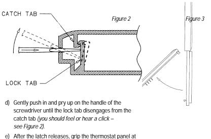
e) After the latch releases, grip the thermostat panel at the bottom corners and swing it up and away from the base to completely separate (See Figure 3).
