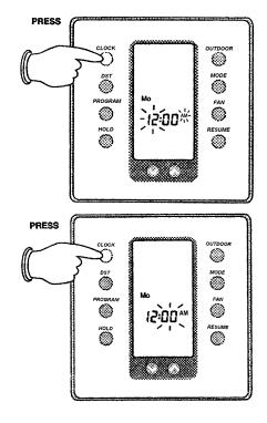
*Step 3*: Press the **CLOCK** button again and "12:" (hours) and "AM" or "PM" will flash. Use the **DECREASE** or **INCREASE** button to change the flashing symbol to the current hour making sure the hour has the proper AM or PM designation.
