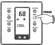
Step 1: Press and release the MODE button until the word "COOL" and the " COOL" cooling symbol appear on the display.
