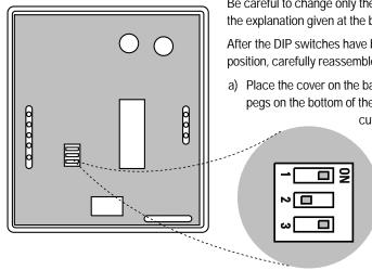
Be careful to change only the intended DIP switches per the explanation given at the beginning of this section.
