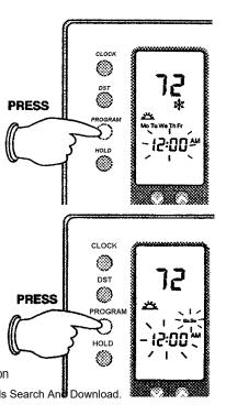
*Step 7:* Press and release the **PROGRAM** button until the temperature for the **Morning** "\_\_\_\_\_" event flashes. Repeat steps 2-4 for the **Morning** "\_\_\_\_\_", **Day** " -\_\_\_\_", **Evening** " \_\_\_\_\_" , and **Night** " ((" events.
