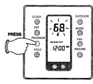
*Step 5:* Press the **DECREASE** button or **INCREASE** button to set the desired minutes for the **Morning** <u>"\_\_\_\_\_"</u> event (program starting times are set in ten-minute increments).
